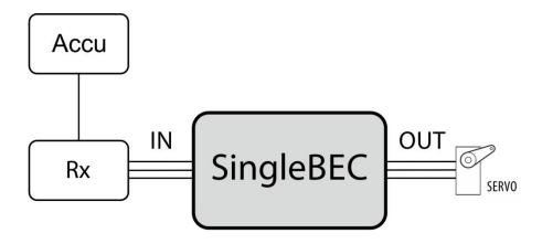
Fig. 1: Application wiring of SingleBEC
