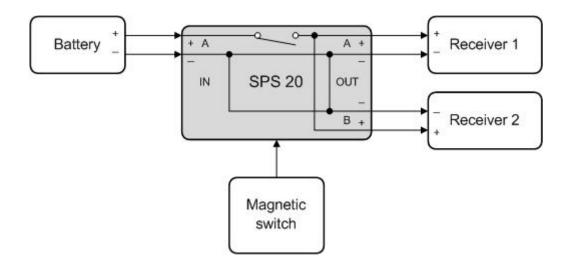
The output current is branched out to two output cable pairs, each pair is able to hold a maximum output transient current of 5A.
