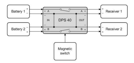
If 2 Batteries are used, "+ poles" batteries mustn't be connected with each other!
