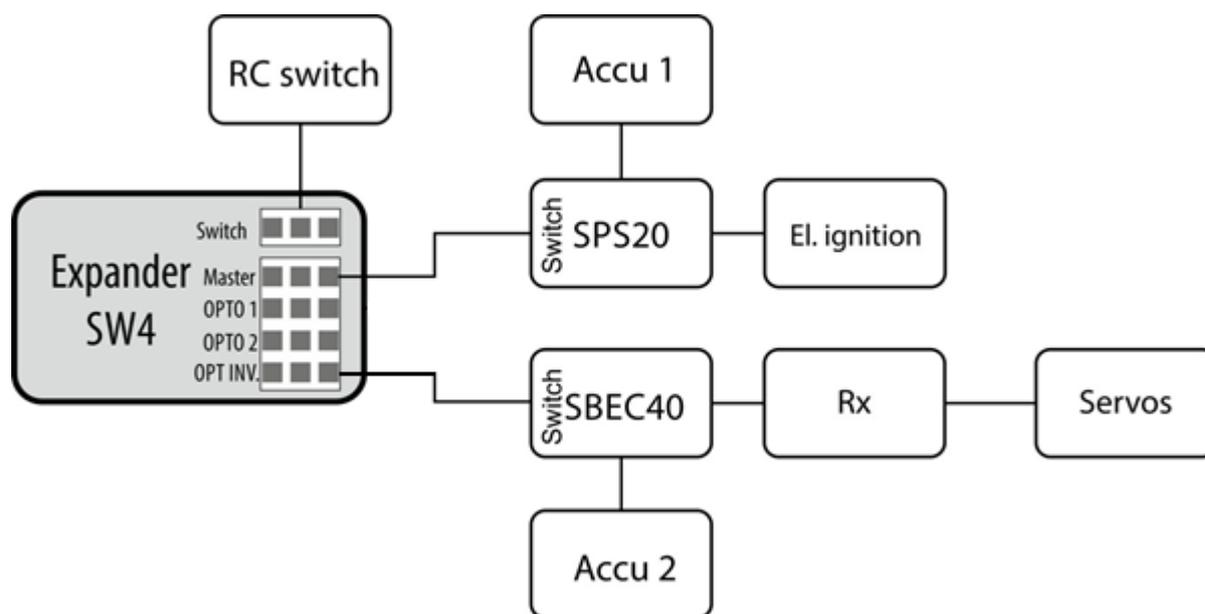
Fig. 1: Expander SW4 application connection
