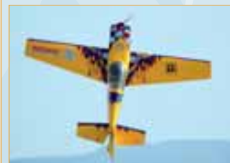
Model EDGE 540 T2 (weight 12,5 kg), with double AXI 5330/20 GOLD LINE
