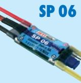
The SP 06 switch carries out switching of auxiliary functions in model airplanes, ships and vehicles, as for instance additional glow plug heating, switching different light systems a.s.o. The switching moment is indicated by flash up of a LED. The SP06 also offers the function of a reverse channel as known from many transmitters. The maximum long-term load of the switch are 6 A and it can be operated within a broad voltage range. Arbitrary voltages between 0,1 V and 15 V can be switched.
