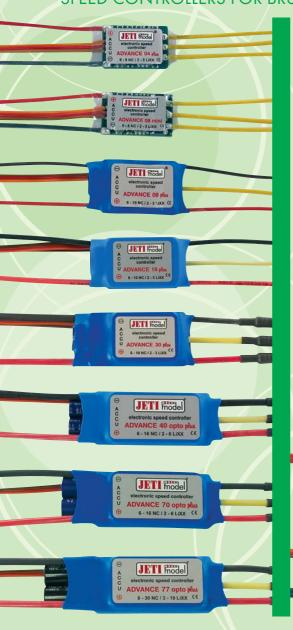
Universal controllers optimized for all types of brushless motor. Jeti plus controllers are suitable for use with NiCd, NiMh, Li–Pol and Li–Ion batteries. The throttle range is automatically set at start up. Brake with hard motor cut off for gliders, or no brake with soft motor cut off can be easily set.
