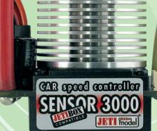
The CAR sensor 3000 controller is designed to control alternating current (brushless BLDC) motors with SENSORS (i. e. only motors which are equipped with rotor position transducers like Hall device sensors or optical sensors) as well as for direct current (DC) motors. As the controller is able to recognize the type of the BLDC motor, its sensor type, and mechanical advance settings, any type of brushless motor with sensors, from any manufacturer, can be connected to it.
