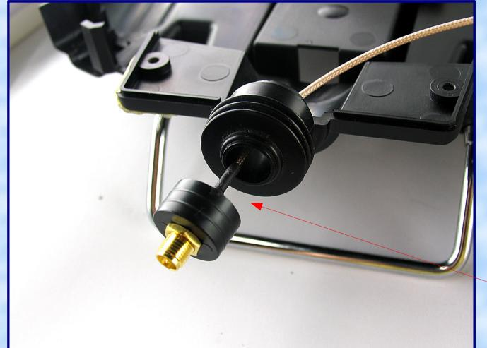
Put connector through out from the transmitter
